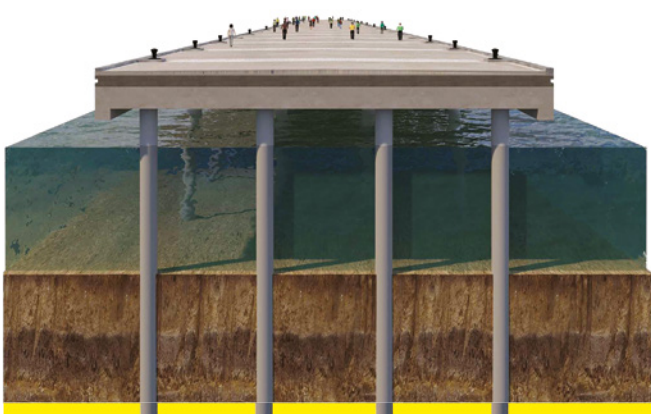
The CBF will be built on pilings allowing water and marine life to flow freely.
