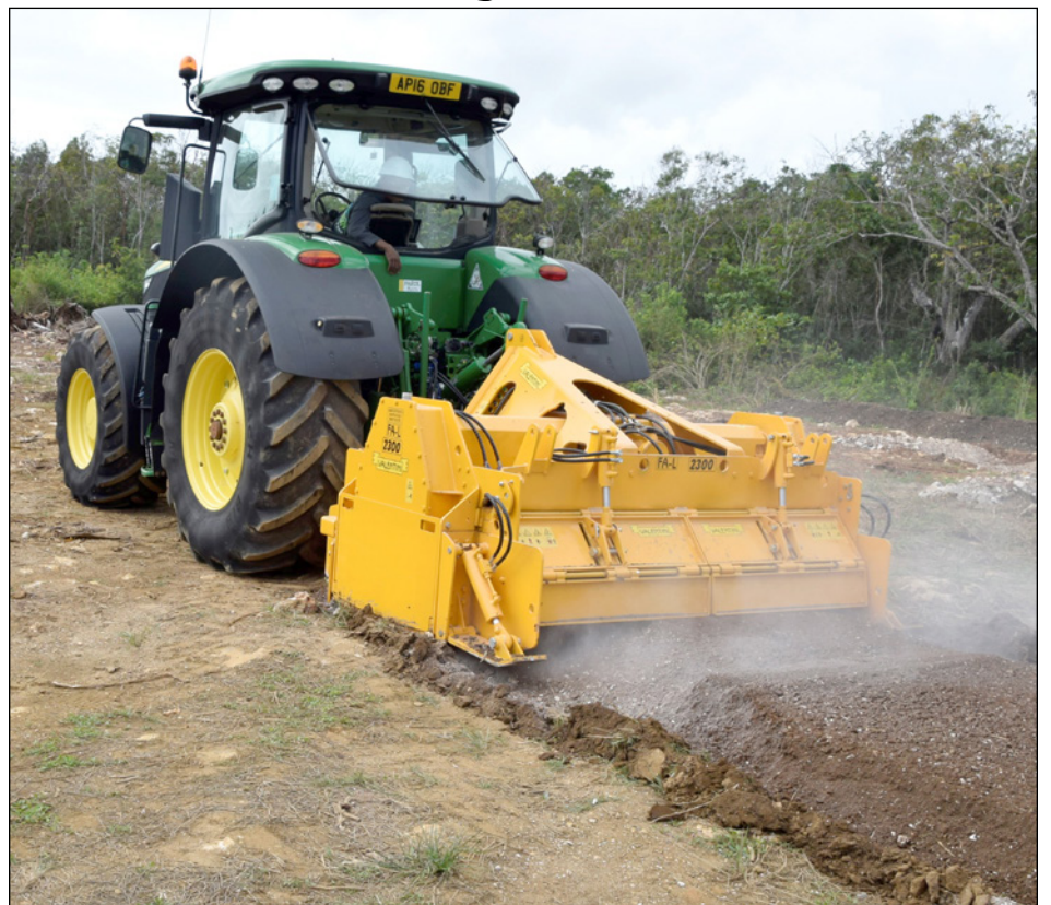
► The new rock-crusher produces usable soil out of rocks
