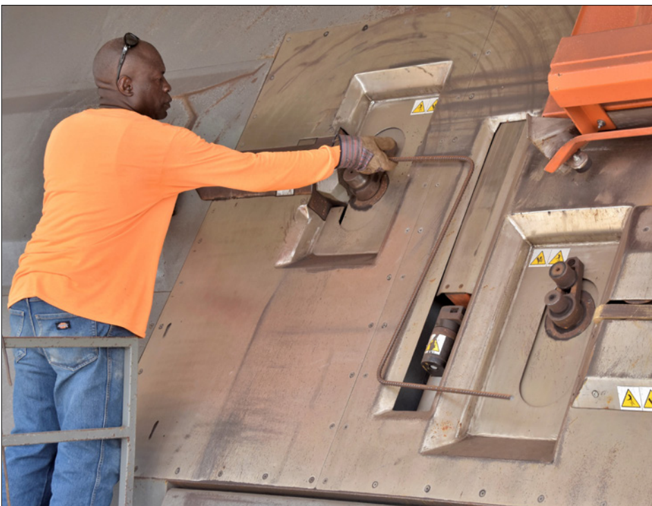
► An employee demonstrates how the rebar can be bent into complex forms, in just seconds
